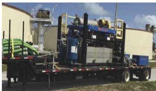
Figure 2. Photos of Pilot Equipment: Thickening (left) and Dewatering (right)
