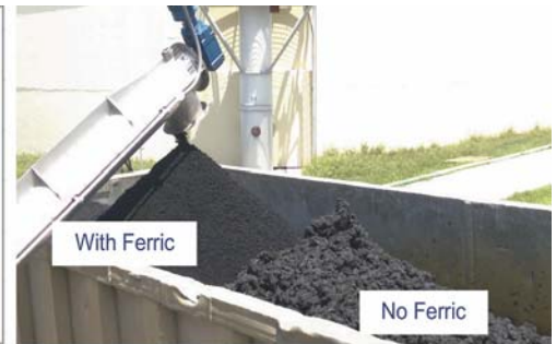
Figure 9. Central District Wastewater Treatment Plant Dewatering Polymer Curve Testing With and Without Ferric Sulfate (data, left; photo of cake, right)
